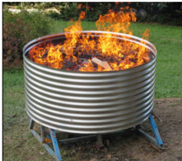
Pyrolysis kiln for the production of biochar based on the principle of the flame curtain ( https://wiki.opensourceecology.org ).
